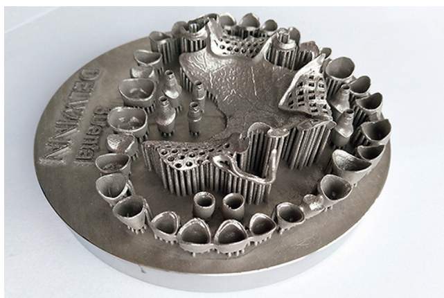
Figure 1. SLM metal copings, removable partial denture framework, and support structure. SLM, selective laser melting.
